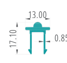
GUIDE RAIL Wt./R.Mtr. : 0.177 kg PART CODE:27021
