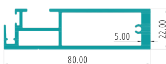
SLIM SGU INTERLOCK (RECTANGLE HURRICANE BAR) Wt./R.Mtr. : 1.448 kg PART CODE:27148
